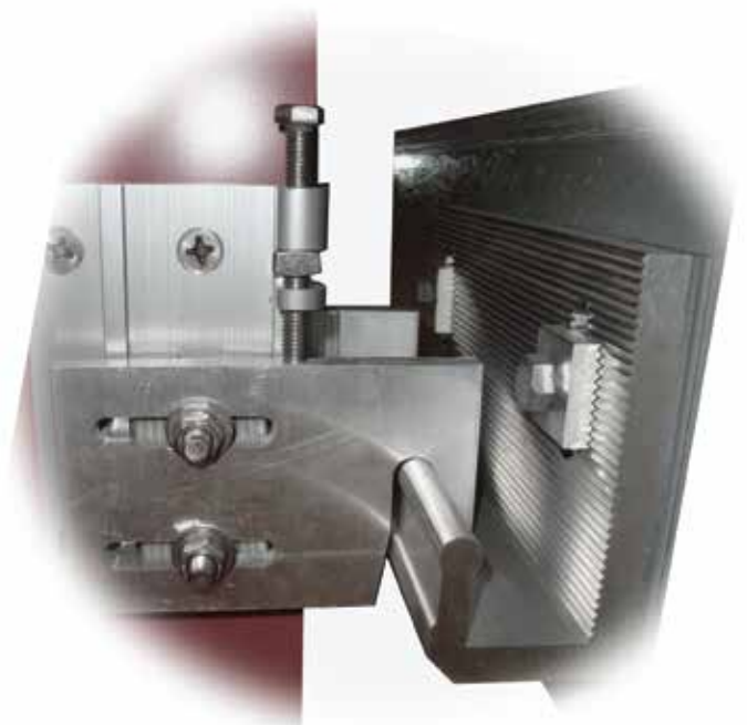
Three-way adjustable “jack bolt” anchor
